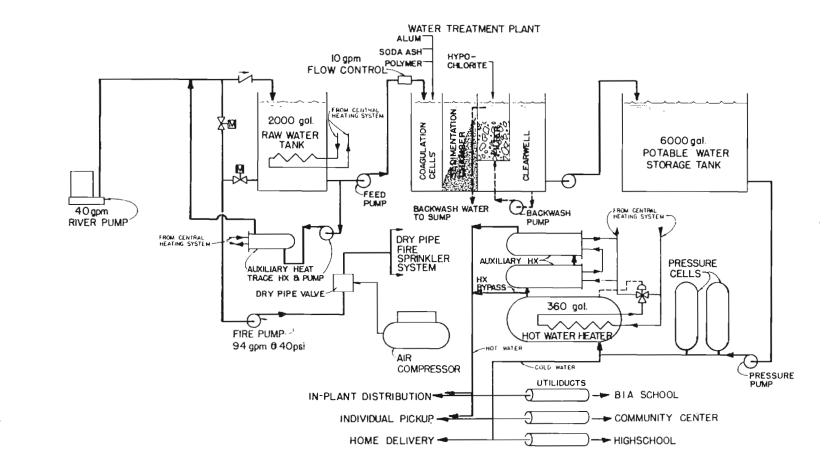
Figure 13. Schematic of water treatment system at Emmonak.
