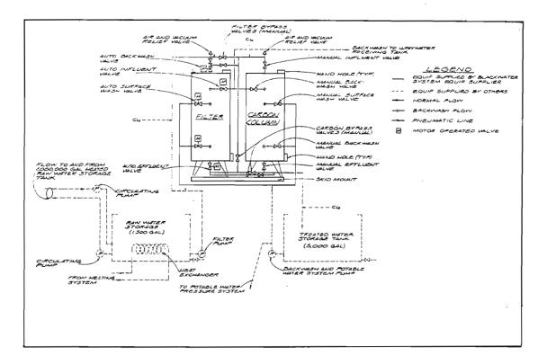
Figure 8. Schematic of water treatment process at Wainwright.
