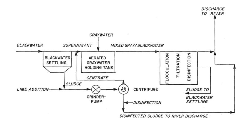
Figure 15. Schematic diagram of modified wastewater treatment system at Emmonak.
